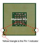
The surface of LGA 775 CPU. Remember to apply some silicone heat transfer compound on it for better heat dispersion.
